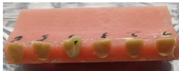
Fig. 8b: Bond of SR Vivdent DCL teeth with Ivobase High Impact. Testing according to EN ISO 22112. Internal measurement, Ivoclar Vivadent.
