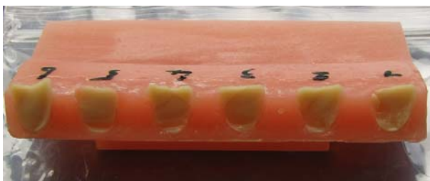
Fig. 8a: Bond of SR Vivdent DCL teeth with Ivobase Hybrid. Testing according to EN ISO 22112. Internal measurement, Ivoclar Vivadent.
