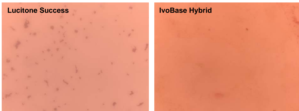
Fig. 14: C. albicans colonization on Lucitone Success and Ivobase Hybrid after 30-minute incubation with prior storage of the specimens in saliva. Considerably more cells had attached to Lucitone Success than to Ivobase Hybrid.
